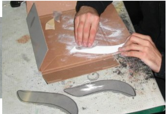
Sand to a polished look. Start with 150, then continue to finish with 250. 400 is for the final work.
