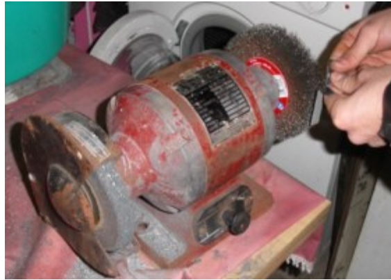
Grind edges to as smooth a finish as you can
