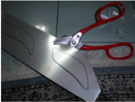
Trace around templates on to sheet metal and carefully cut out.
